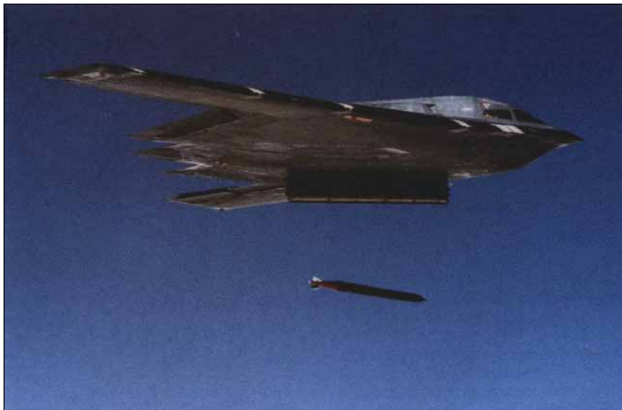
USAF continues to test various weapons with its B-2 Spirit stealth bomber, which achieved IOC April 1. In a February test, a B-2 dropped a 4,700-pound GAM-113 at China Lake NAWC, Calif. Northrop Grumman and Hughes Aircraft developed the near-precision, deep-penetration GAM-113, which the Air Force said is effective against deeply buried hard targets.
