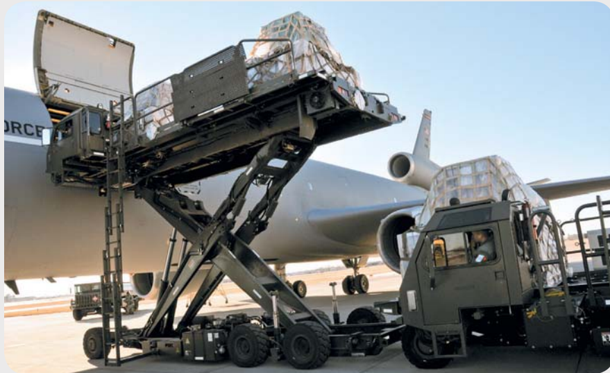
Left: Halvorsen in 1989 leans out of the window of a C-54 on static display at Tempelhof. After coming home and earning two engineering degrees, the Candy Bomber went back to Berlin to take charge of the air base for USAF. Below: A Halvorsen Loader lifts relief supplies for Afghans onto a KC-10. The massive 25,000-pound loader was named in honor of Halvorsen in 2001.
