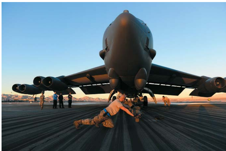
Carefully, Carefully: SrA. John Myer positions a tow bar under the tire of a B-52 during a Red Flag exercise at Nellis AFB, Nev. The massive bomber shredded a tire landing after a Red Flag mission Feb. 1.
