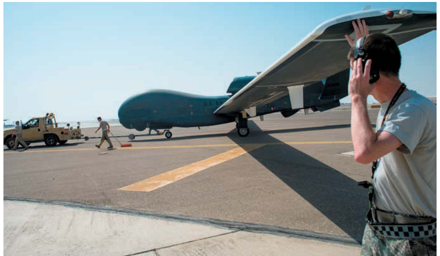
Airmen complete postflight checks on an RQ-4 Global Hawk in Southwest Asia. Specially equipped Global Hawks are proposed as a solution to communications hurdles between F-22 and F-35 aircraft.
