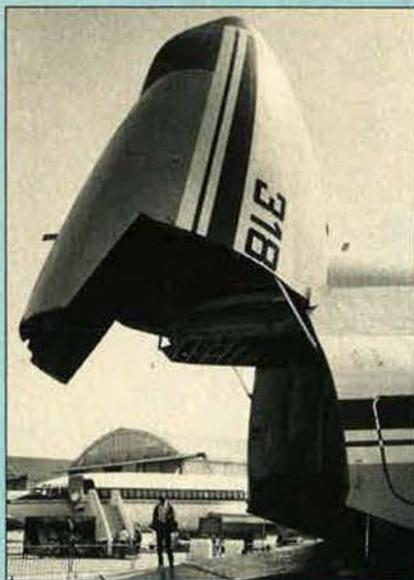
As on Lockheed's C-5 Galaxy, the Antonov's visor nose opens upward around the flight deck (Air Portraits)
