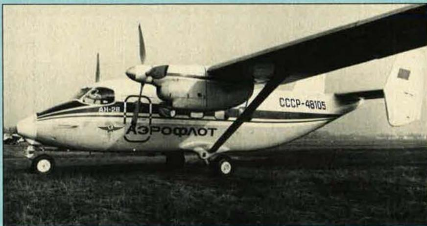
Antonov An-28 light general purpose transport (two Glushenkov TVD-10B turboprop engines)
