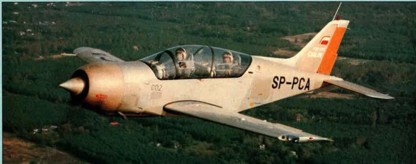
First flying prototype of the PZL-130 Orlik trainer (Vedenyev M-14Pm radial piston engine)
