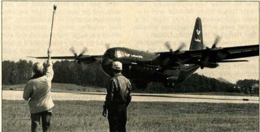
*Lockheed-Georgia Company's High Technology Test Bed Aircraft (HTTB) has set three time-to-climb records for short takeoff and landing aircraft, including reaching 31,000 feet in 17.7 minutes. Man in foreground measures wind speed.*
