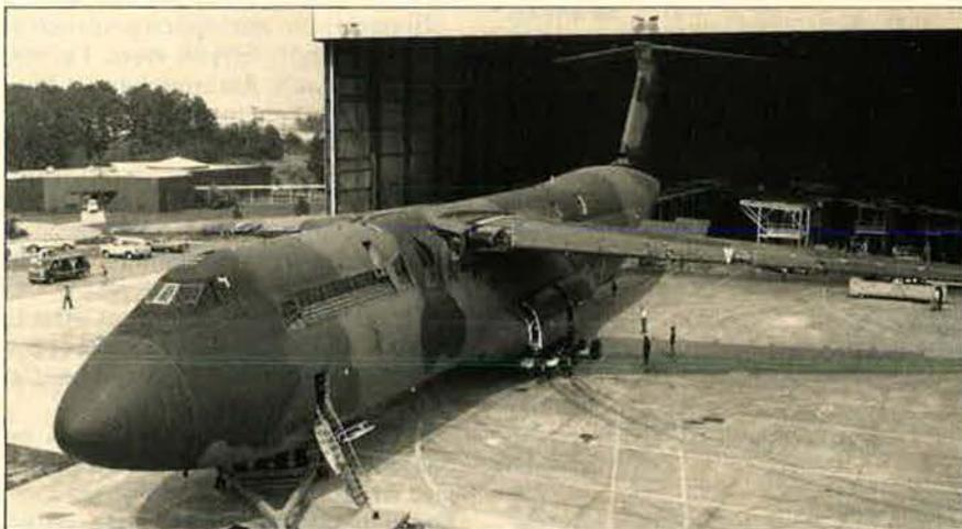
*The first of Lockheed's giant new C-5B Galaxy military transports, after installation of its wings, is moved to the final assembly position so the four General Electric engines can be mounted. USAF is buying fifty C-5Bs.*
