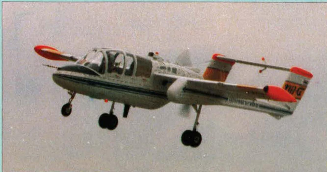
First flights of the RTAF-5 were made with the landing gear fixed in the down position
