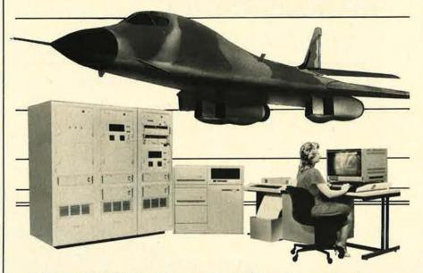
FSI's DYNAMIC SCENARIO THREAT GENERATORS provide the full frequency range of threat emitters to the B-1B AN/ALQ-161 Defensive Avionics System in systems integration tests at Eaton Corporation and at Edwards Air Force Base. Realistic threat systems and pulse doppler emitter signals are dynamically varied in precise time and space as the B-1B is electronically "flown" by FSI's Combat Systems Simu-
