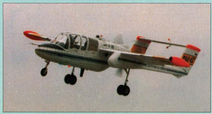
First flights of the RTAF-5 were made with the landing gear fixed in the down position
