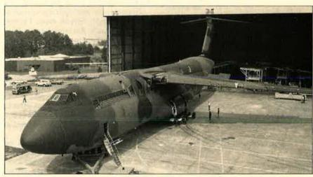
The first of Lockheed's giant new C-5B Galaxy military transports, after installation of its wings, is moved to the final assembly position so the four General Electric engines can be mounted. USAF is buying fifty C-5Bs.
