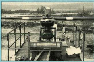
GEC Avionics Phoenix battlefield surveillance and target acquisition RPV on its launching ramp
