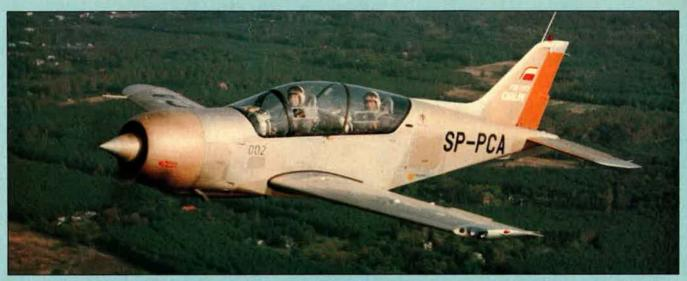
First flying prototype of the PZL-130 Orlik trainer (Vedeneev M-14Pm radial piston engine)
