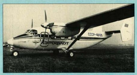
Antonov An-28 light general purpose transport (two Glushenkov TVD-10B turboprop engines)
