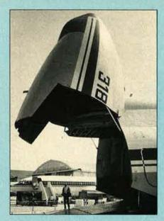
As on Lockheed's C-5 Galaxy, the Antonov's visor nose opens upward around the flight deck (Air Portraits)
