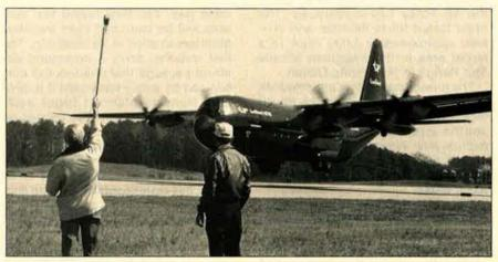
Lockheed-Georgia Company's High Technology Test Bed Aircraft (HTTB) has set three time-to-climb records for short takeoff and landing aircraft, including reaching 31,000 feet in 17.7 minutes. Man in foreground measures wind speed.
