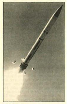
On April 20, the Army's Flexible Lightweight Agile Guided (FLAG) Experiment Program hypersonic test vehicle, shown above at launch, destroyed an aluminum sphere suspended below a balloon at 15,000 feet. The FLAG program is part of the SDI effort.
