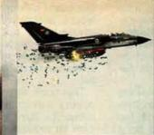
MW-1. Multipurpose weapon system to be used on the Tornado.
