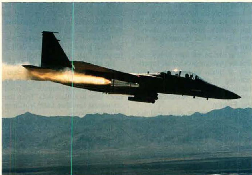
An F-15E dual-role fighter launches an AGM-65B TV-guided Maverick missile designed mainly for destroying enemy tanks. Under heavy budgetary pressure, USAF decided early last year to buy only about half of its originally planned number of F-15Es. Champions of the aircraft are pushing to reverse that decision.
