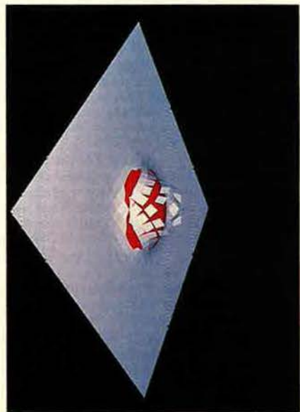
In a series of three-dimensional, computer-generated images created with DYNA3D, a rigid ball breaks through a steel plate. The structural analysis program can simulate any kind of metal stress, from pressure to impact to chemical blast.
