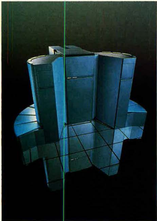
DYNA3D uses some 100,000 equations to simulate a car crash. Running a crash takes fifteen to twenty hours on a Cray X-MP-42 supercomputer. Its successor, the Cray Y-MP pictured here, will be used to model crash effects on vehicles and their occupants at the same time.
