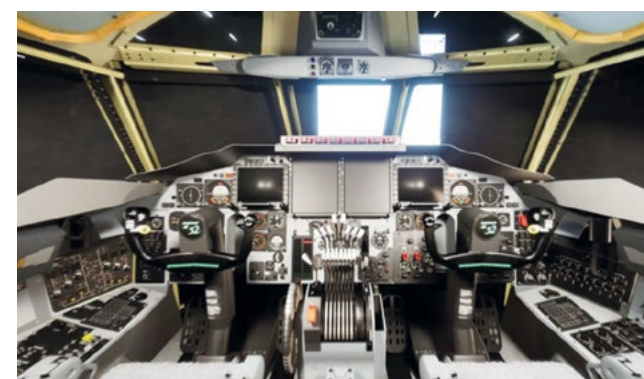
B-52H's likely future cockpit, after radar and engine modifications have been made to the 60-year-old bomber, as shown in a Boeing graphic.
