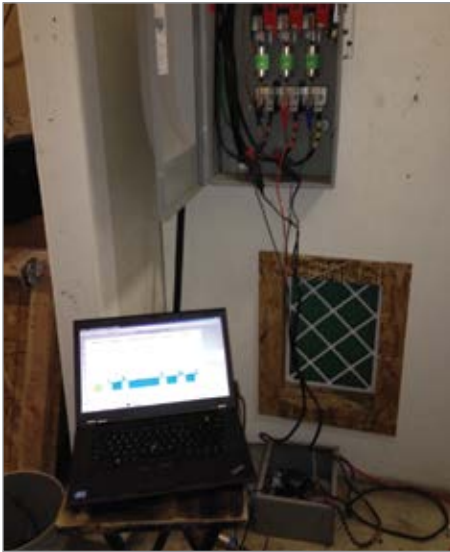
Figure 2: Downloading performance metrics from the data loggers provides helpful charts for the end user.
