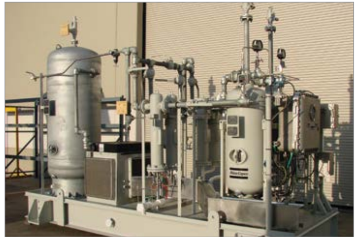
Instrument air CDE 250+ skid package included a sandstorm protection package. Components included a wet air receiver tank, auxiliary cooler, water separator, duplex air pre and after filters with a nine (9) valve by pass system and a heatless regenerative desiccant air dryers.
