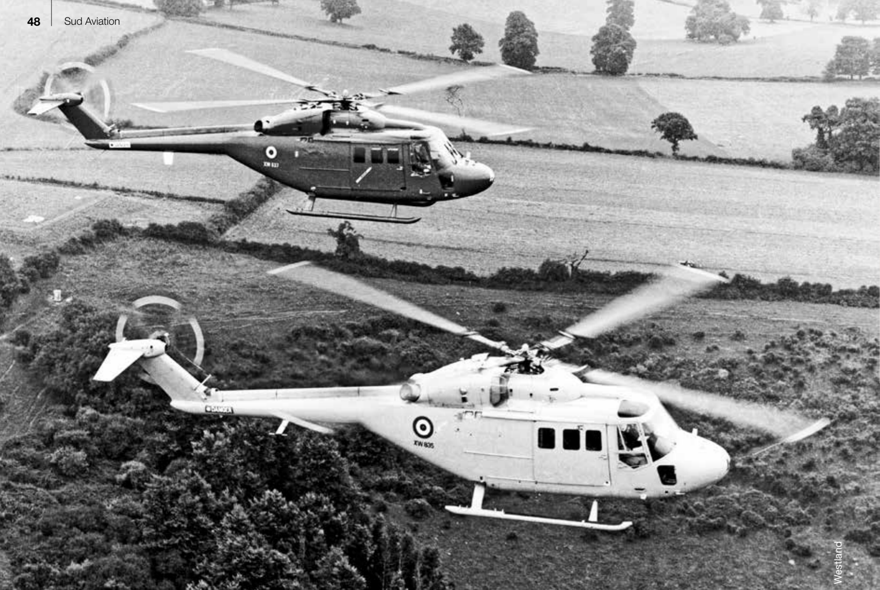
The WG13 Lynx, the all-titanium rotor hub of which was manufactured at Marignane.
