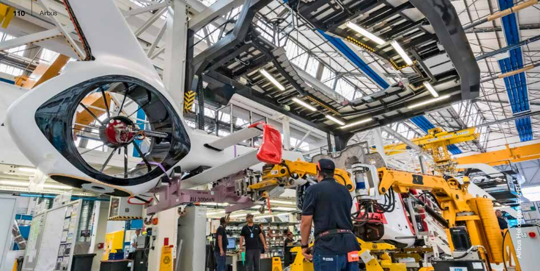
The H160's final assembly line entered into service in January 2018.
