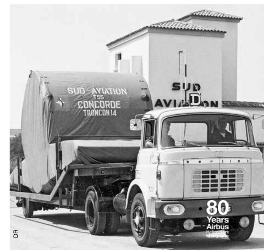
Shaft section 14 had a more complex structure than shaft section 12 as it was to include the fuse of the wing.
