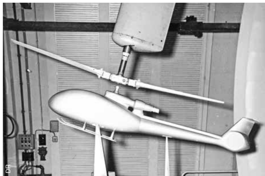
First test of the Fenestron® in the wind tunnel in April 1967.
