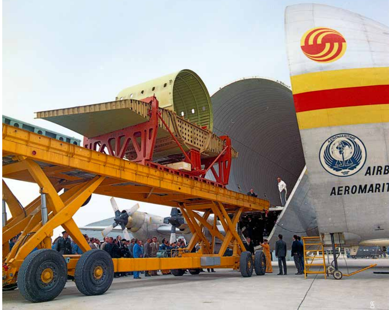
The shaft sections were loaded into the Super Guppy, specially chartered for this occasion, to be transported to Toulouse where the assembly line was based.
