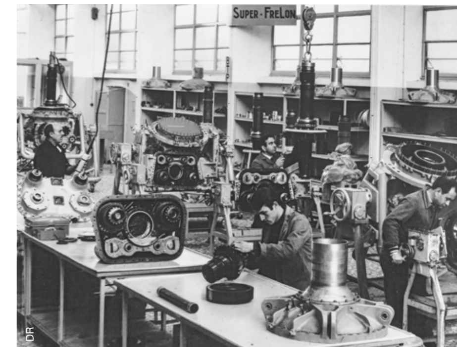
Assembly of the Super Frelon mechanical systems.
