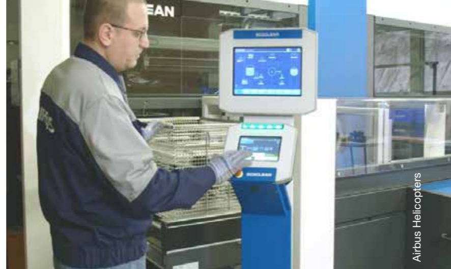
«Eccoclean™» machine for eliminating machining dust and residue before packaging.
