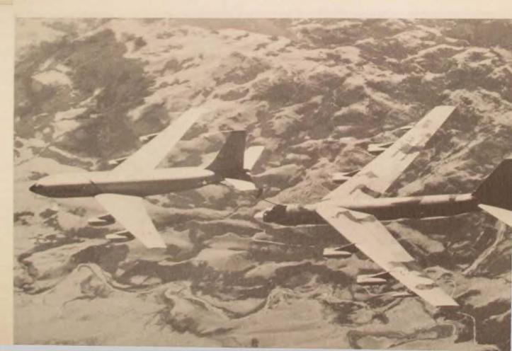
program for all SAC KC-135s that incorporates new jet engines and replaces or modifies 25 other systems or subsystems. The program increases off-load capability by 50 percent, improves fuel efficiency by 27 percent, significantly enhances reliability, and extends the useful life of the KC-135 far into the next century.
