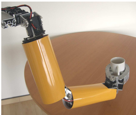
Fig. 3. 7 DOF human-scale anthropomorphic arm with 2 DOF gripper.
