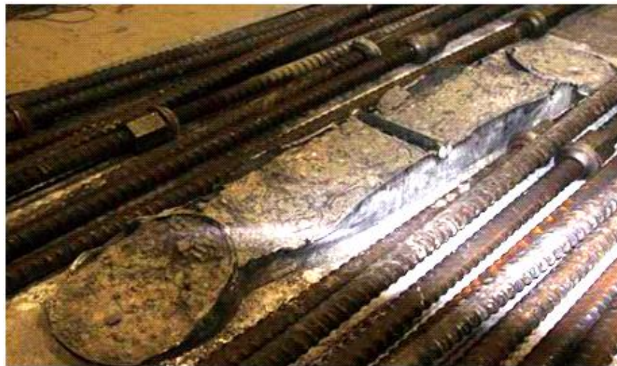
Figure 5-66 Cut Base of Specimen CFSSP-B2 After Testing
