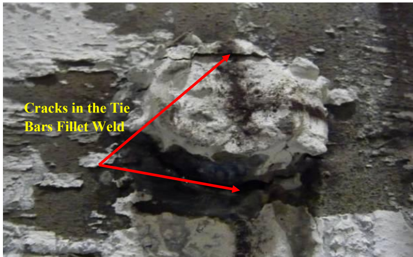
Figure 5-59 Cracks in the Tie Bar Fillet Welds of CFSSP-B2 at 3.33% Drift
