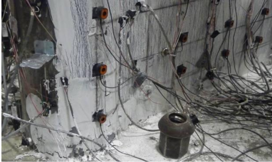
Figure 5-53 South West View Specimen CFSSP-B2 at 1.33% Drift
