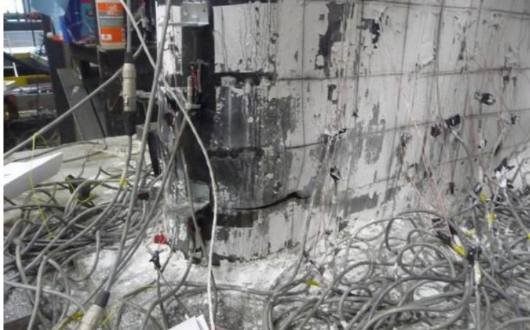
Figure 5-31 Fracture Propagated in the HSS part of Specimen CFSSP-NB2 at 3.0% Drift
