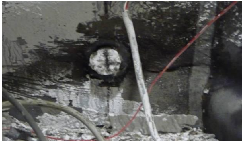
Figure 5-64 Propagation of Crack from Web to HSS of Specimen CFSSP-B2 at 4.67% Drift
