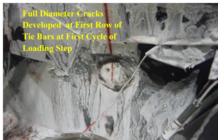
Figure 5-10 Specimen CFSSP-NB1 Tie Bars Plug Welding Cracks at 2.4% Drift
