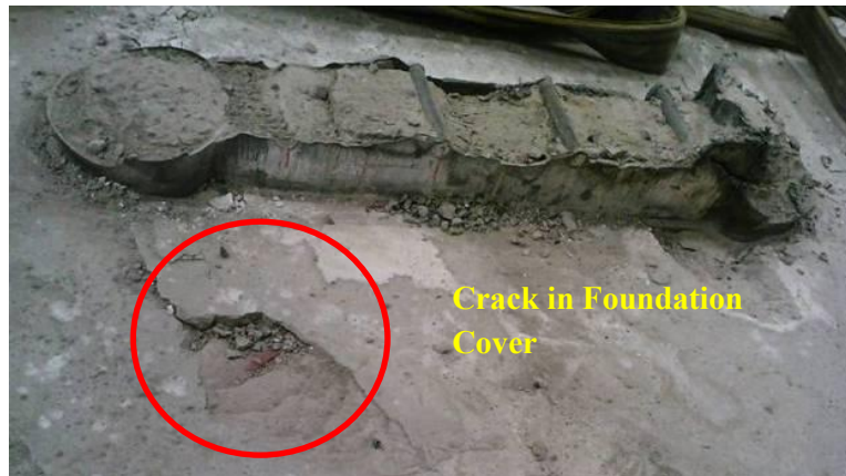
Figure 5-49 Cut Base of Specimen CFSSP-B1 After Testing
