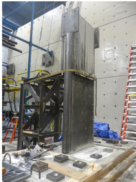
Figure 4-28 Specimen CFSSP-NB1 After Concrete Pouring
