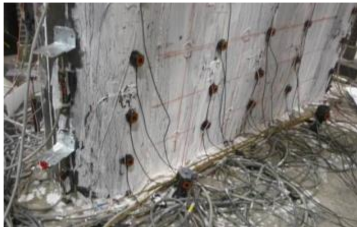
Figure 5-38 South West View Specimen CFSSP-B1 at 1.33% Drift
