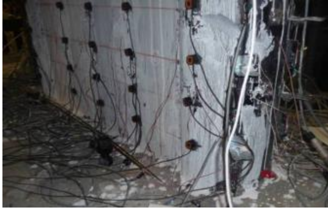
Figure 5-37 South East View of Specimen CFSSP-B1 at 1% Drift
