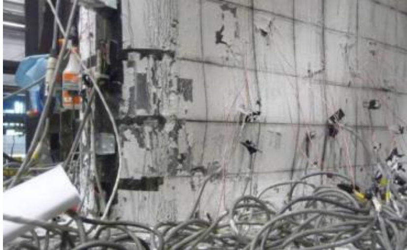
Figure 5-25 First Wave of Local Buckling Specimen, South East Side, CFSSP-NB2 at 1.8% Drift
