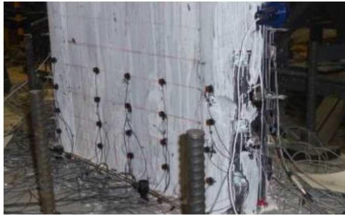
Figure 50-36 South West View of the Specimen CFSSP-B1 at 0.67% Drift
