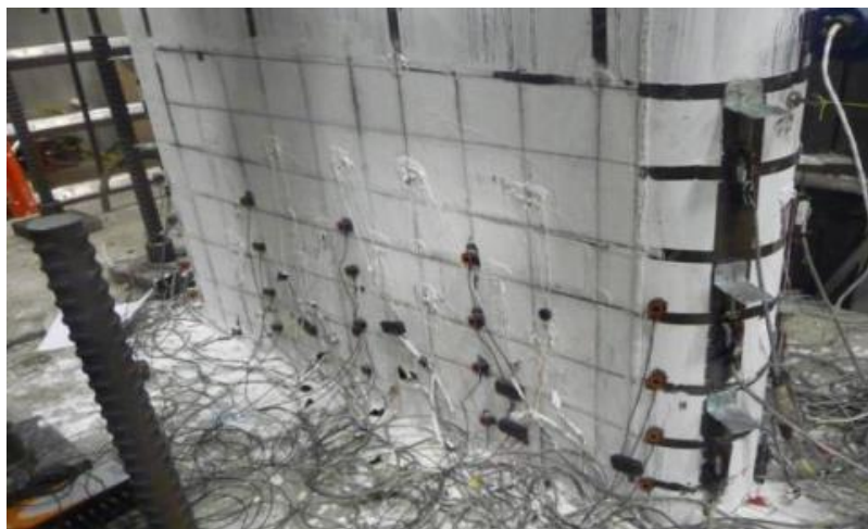
Figure 5-20 North West View for Specimen CFSSP-NB2 at 0.4% Drift
