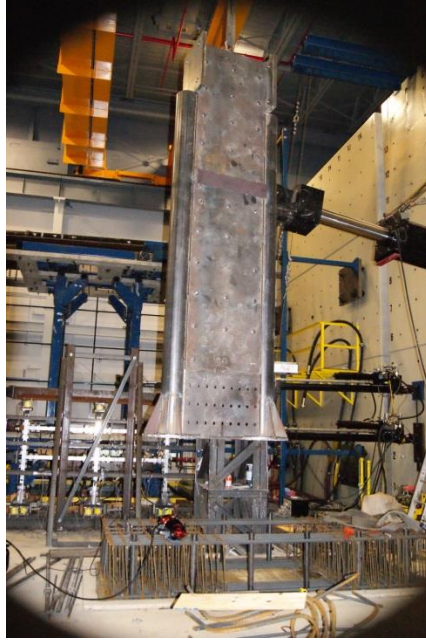
Figure 4-23 Setting CFSSP-Wall in Position
