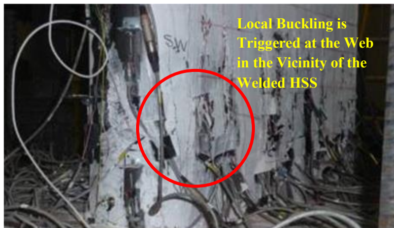
Figure 5-7 South West View for Specimen CFSSP-NB1 at 1.8% Drift
