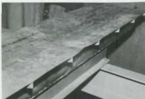
Fig. 11. View of model II destroyed by loading scheme B.
