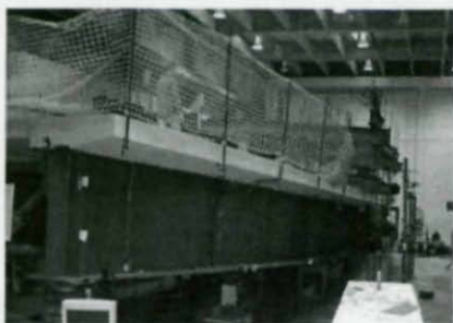
Fig. 4. View of deformed composite test bridge slab along G3 just prior to the concrete slab crushing (Courtesy of Federal Highway Administration)
