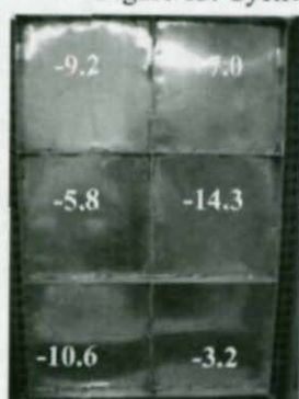
Figure 14: Real (a) and numerical (b) deformed shape for panel type B.
