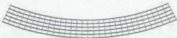
Figure 4 – Plan View of Finite Element Model
