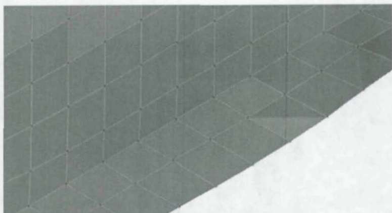
Figure 9 25 mm (1 in) shell finite element mesh of the test model flange-web junction displaying full nodal continuity along the entirety
