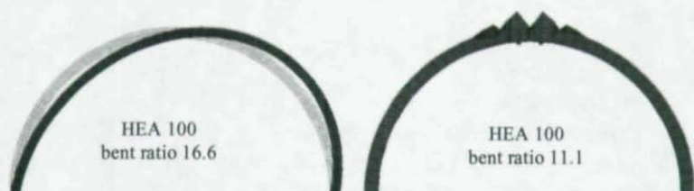
Figure 6. Arch buckled in sway mode and in local flange buckling.
