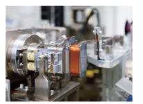
High-density coil winding machine for motors
