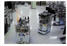
This system obtains the production status, the operation status of automated guided vehicles (AGVs), etc. in real time to generate and distribute the optimal conveyance plan based on the obtained information, thereby achieving autonomy conveyance with AGVs.
