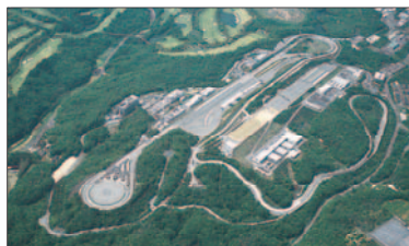
Fujioka Proving Ground (completed 1970) Location: Mitsukuri-cho, Toyota-shi, Aichi Prefecture Area: approx. 670,000 m 2 Flat circumference: 2.4 km; Poor road circumference: 4.6 km
