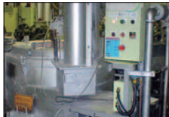
Improvements in facilities Reducing fuel in die-cast aluminum molten holding furnaces employing heat exchange integrated burners
