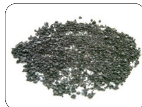
Conversion of waste plastic and sludge into molten slag, used as subbase material
