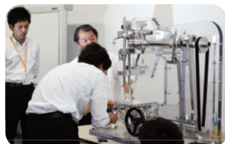
Mock-up sewing machine three times the ordinary size with a transparent plastic cover.
