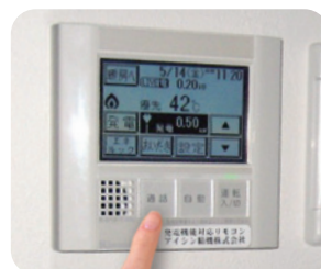
Kitchen remote control device for the Coremo prototype installed for trial use. Amount of power generated, CO 2 reduction and cost-saving data can all be viewed.
