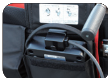
The connector and battery can now be connected from the seated position
