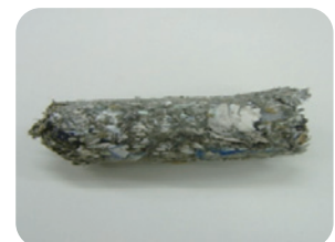
Conversion of waste plastic into RPF* used as fuel for boilers
