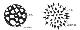
Fig. 2 Muskmelon-form and *kompeito*-form  $TiO_2$  photocatalytic particles.
