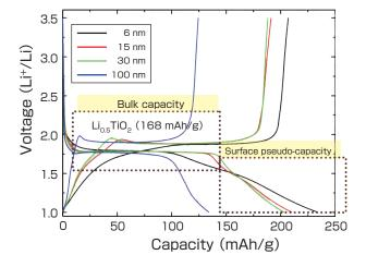
Fig. 6 Charge-discharge curve of nanocrystalline titania.
