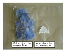
Photo 7. TiO<sub>2</sub> deoxidant before absorbing oxygen (blue) and after absorption (white).
