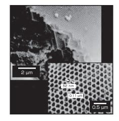
Fig. 5 Titania nanoporous electrode.
