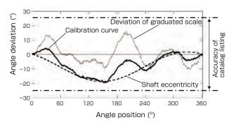
Fig. 3 Example of deviation factors in calibration curve.
