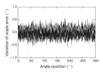
Fig. 11 Reproducibility of calibration value of rotating table (dynamic angle deviation).
