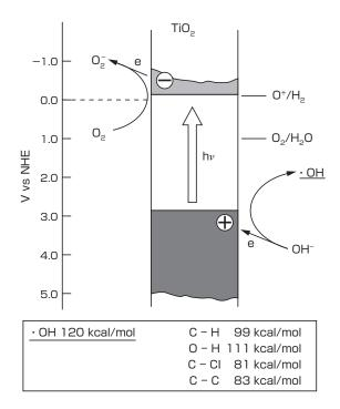
**Fig. 1 Energy level and photocatalysis of titanium dioxide.** V = electrical potential, NHE = normal hydrogen electrode. V vs. NHE is potential against normal hydrogen electrode, or potential when normal hydrogen electrode is used as standard. h  $\nu$  = energy of light.
