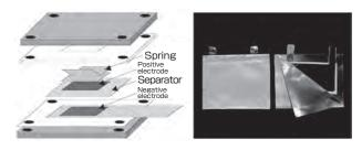
Fig. 9 Structure and photograph of laminated battery cell prototype.
