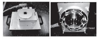
Fig. 8 Rotating table equipped with self-calibratable rotary encoder "SelfA".
