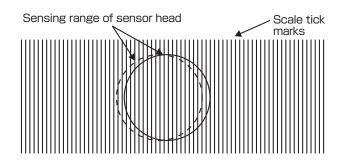
Fig. 13 Scale measurement size of rotary encoder.
