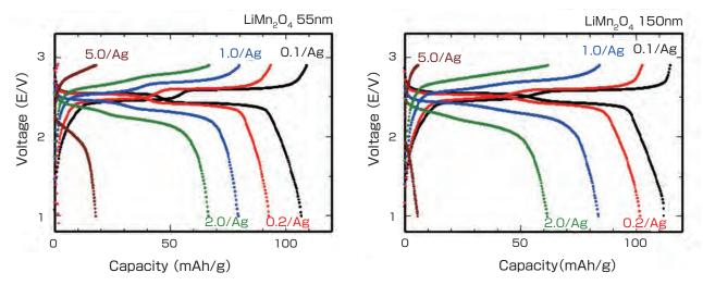
Fig. 10 Output property of lithium battery using nanocrystal electrode.
