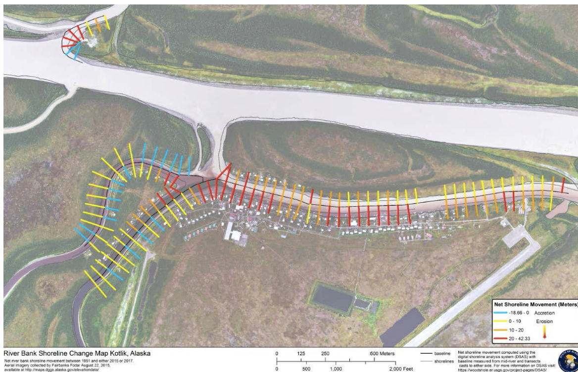
Figure 10: Preliminary riverbank shoreline change map of Kotlik showing the net shoreline (riverbank) movement from 1951 to either 2015 or 2017 (where data is available). Hot colors show areas of erosion and blue shows accretion. Created by DGGs, Jacquelyn Overbeck, Jacquelyn.overbecak@alaska.gov in 2017.
