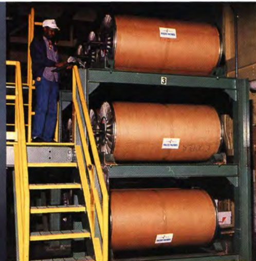
Warp beams for tire cord fabrics in Scottsboro, Alabama.
