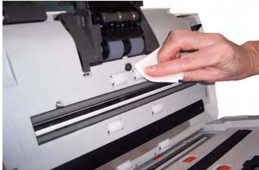
*IMPORTANT: The roller cleaning pad contains sodium lauryl ether sulfate which can cause eye irritation. Refer to the MSDS for more information.*
