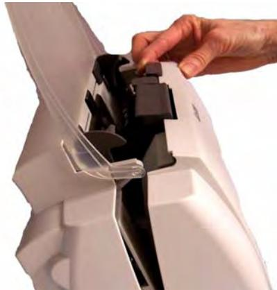
3. When you finish cleaning the scanner or replacing a part, close the scanner cover with both hands.
