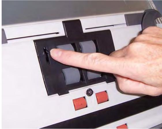
1. Lift the tab of the feed module cover and remove it from its position.
