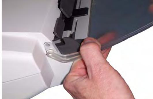
1. Push the separation module up to snap out and lift it out of position.
