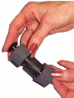
5. Install each new tire by gently pulling it over the core.
