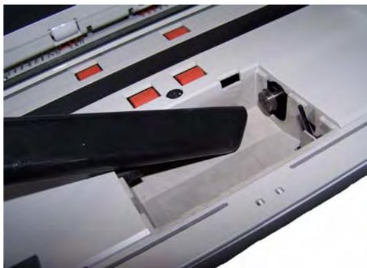
6. Reinstall the feed module by aligning the pins and pushing it toward the left to fit it into position. Be sure the gears are aligned and it snaps into place. Roll the feed module back into place.
