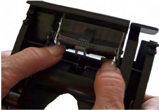
3. Push down on the side tabs until the pre-separation pad protrudes slightly from the front of the separation module.
