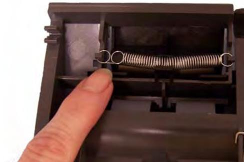
3. Lift the spring from the holder and move it to the left or right as desired to adjust the tension.
