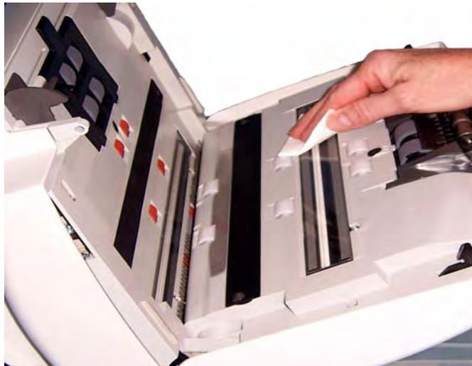
2. Wipe the upper and lower imaging area again using the reusable optics cleaner pad to remove any streaks.
