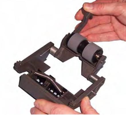
3. Remove the separation roller from the separation module housing.
