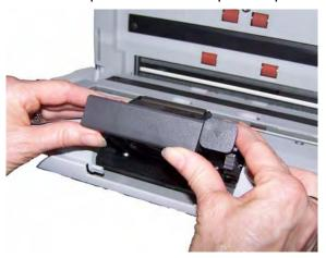
2. Manually rotate and wipe the separation module tires with a roller cleaning pad.
