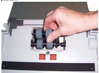
3. Manually rotate and wipe the feed module tires with a roller cleaning pad.
