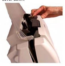
3. When you finish cleaning the scanner or replacing a part, close the scanner cover with both hands.
