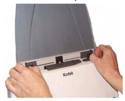
4. Adjust the input tray. You can scan documents with the input tray open or closed. Feed documents with the input tray open if you are scanning a batch of documents.
