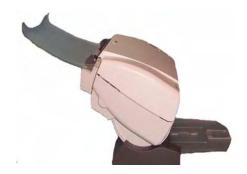
Upright position: Use this position if you are scanning in tight spaces. Press and hold the tilt button and rotate the scanner toward you.
