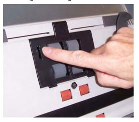
1. Pull against the raised edge of the feed module cover and lift it up and out of position.
