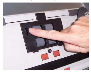
1. Lift the tab of the feed module cover and remove it from its position.
