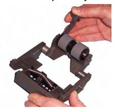
3. Remove the separation roller from the separation module housing.
