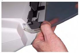
1. Push the separation module up to snap out and lift it out of position.
