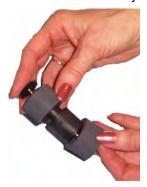
5. Install each new tire by gently pulling it over the core. *IMPORTANT:Do not overstretch the tire; it may tear.*
