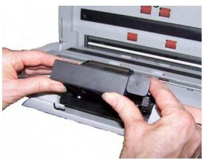
If you are replacing the separation module, insert the new separation module by aligning the tabs with the slots and snapping it into position.
