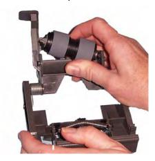
4. Remove each tire by sliding the tire off the core.
