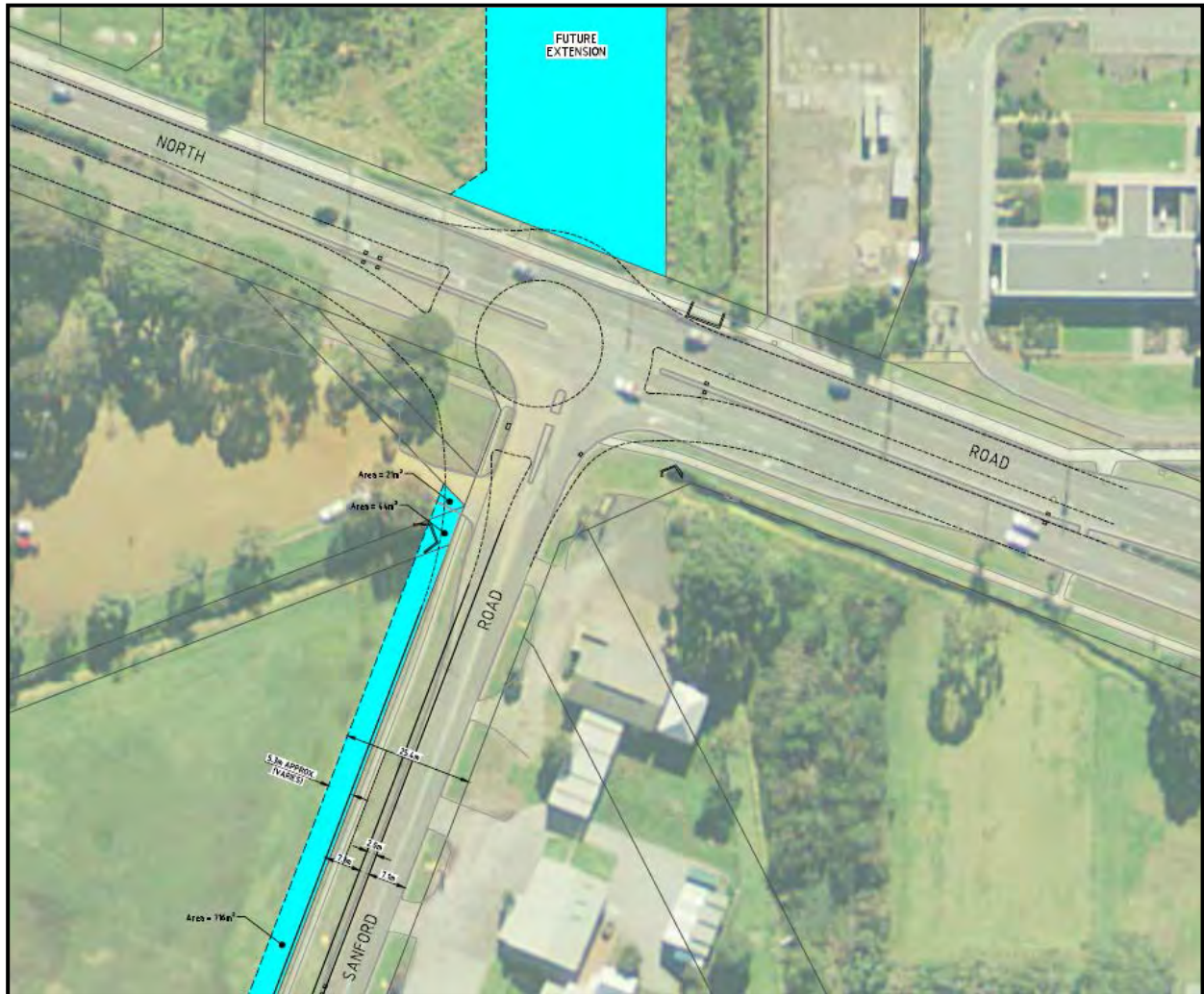
FIGURE 19. RANGE RD TO NORTH RD – INTERSECTION DESIGN
