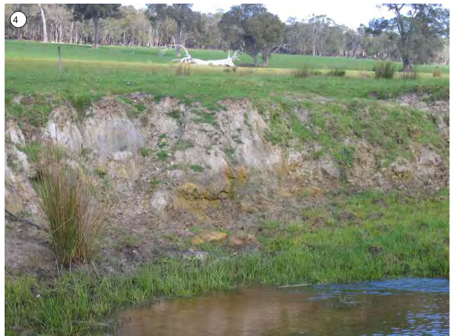
Section of creek line showing sand over yellow silty clay at depth
