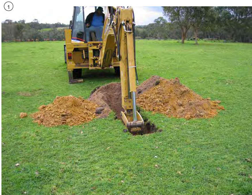
Light brown sand over yellow silty clay that is common across the site and typical of better drained areas
