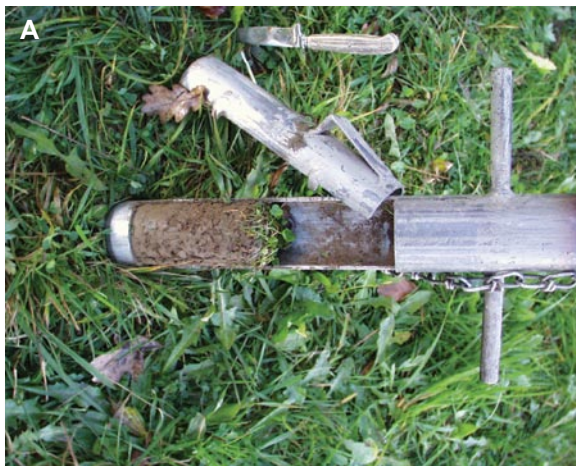
Photo 29.8. Soil corer (A) used to collect microdriles (especially Enchytraeidae) and an example of a forest soil sample (B). (Photos J. Römbke)
