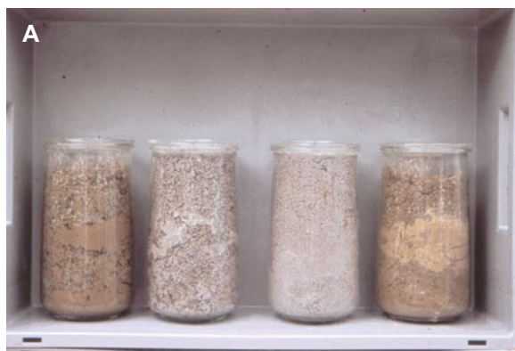
Photo 25.1. Test vessels of the Acute Test (A). Grey: OECD artificial soil; Brown: field soil. Eisenia fetida on the surface of a test vessel (B). (Photos J. Römbke)
