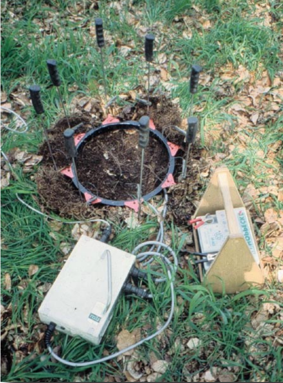
Photo 29.1. Oktet earthworm electrical sampling method developed by Thielemann (1986). The photo shows the eight electrodes, the battery and the control module box. (Photo J. Römbke)
