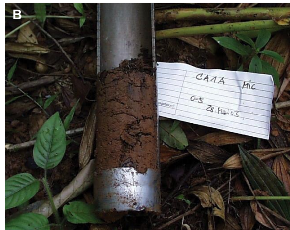
Photo 29.8. Soil corer (A) used to collect microdriles (especially Enchytraeidae) and an example of a forest soil sample (B). (Photos J. Römbke)
