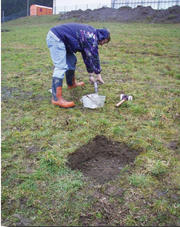
Photo 29.2. Digging of a hole (50 * 50 cm) for earthworm sampling. (Photo J. Römbke)
