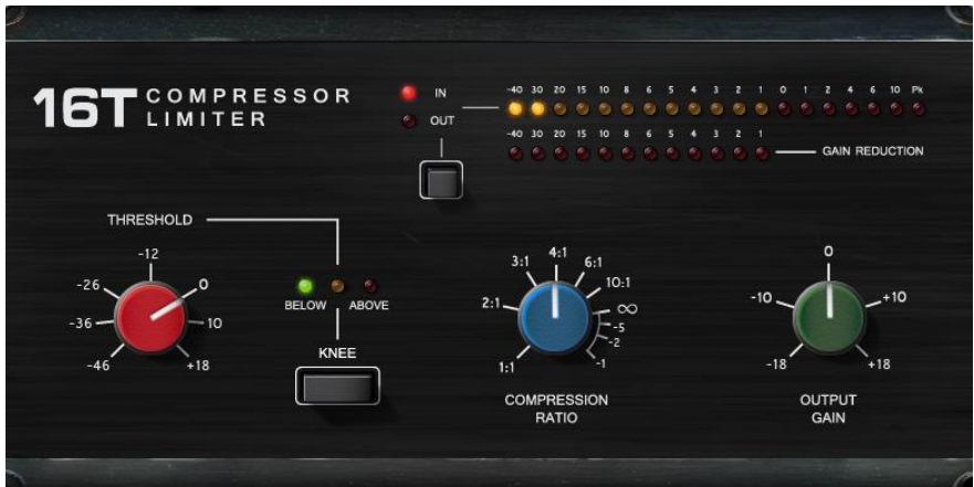
16T - Inspired by an industry classic VCA based RMS compressor this model produces a tight, punchy compression particularly useful with live bass and percussion and also vocals, and with a very easy to use three rotary control interface.
