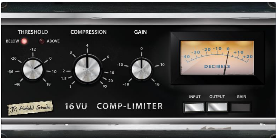
16VU - Based on an original vintage VCA based RMS compressor with VU needle meter, with pleasant characteristic sound due to its non-linearity and distortion artefacts, and also with a simple three rotary control interface.
