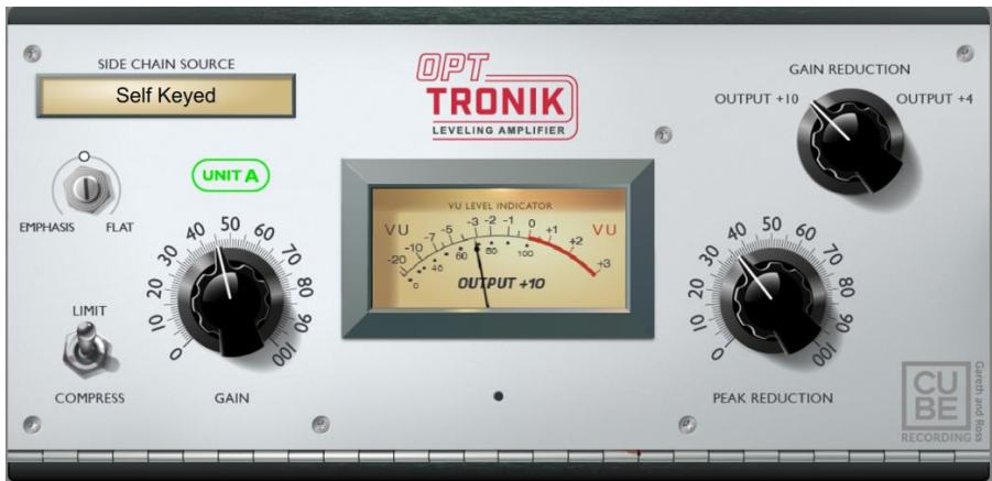
OptTronik – Based on a legendary tube-driven, electro-optical compressor, OptTronik offers smooth, musical compression with easy to use controls. The Limit/Compress switch is used to set the compression ratio and amount of compression is determined by the Peak Reduction control. The Gain control can be used to restore any volume lost to compression. The Emphasis control is used to set the high frequency response of the compressor.
