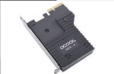
The Eisblock HDX-2 for one M2 SSD - passive cooled
