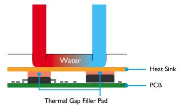
In areas where space between surface is uneven or varies and where surface textures are a concern regarding efficient thermal transfer, the supple consistency of Gap Filler Pad is excellent for filling air gaps and uneven surfaces.
