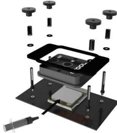
Mounting the cooler on an AMD Socket AM2 - AM3 + CPU
