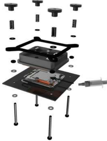
Mounting of the cooler onto an Intel socket 775 - 1156 CPU
