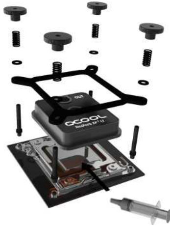
Mounting the cooler on an Intel Socket 2011 CPU
