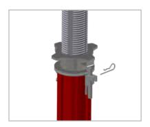
Extraction of the folding pin reassuring securing the bolt.
