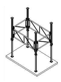
**N.B.**: Maximum bearing capacity for towers with the following dimensions : 2300 x 1500mm and 1500 x 1500mm.
