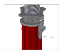
Pressure on the spring bolt for liberation of the nut.
