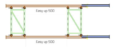
Forming the tower Now install the lattice girders to complete the rectangular shape of the tower.
