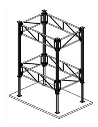
**N.B.**: Maximum bearing capacity for towers with the following dimensions:  $2300 \times 1500 \text{mm}$  and  $1500 \times 1500 \text{mm}$ .
