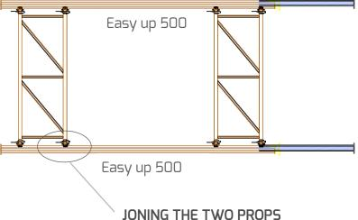
Join the first two props laid on the ground with the lattice girders
