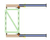
The second pair of easy props Position the props on the lattice girder heads and fasten them.
