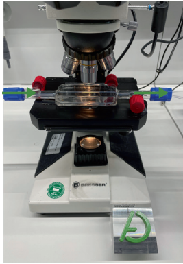
Fig. 2: Setup of the measurement flow cell for optical accessibility of the emulsification process.
