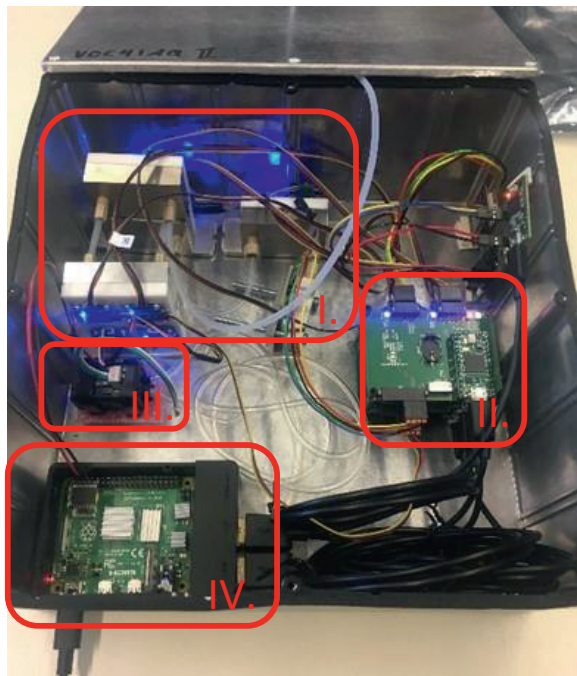
Fig. 2: Inner view of the benchmark system with MOS sensors in measuring chambers (I), control hardware (II), pump (III) and Raspberry Pi for control and data storage (IV).
