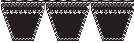
Envelope 5V, 8V Cross Section
