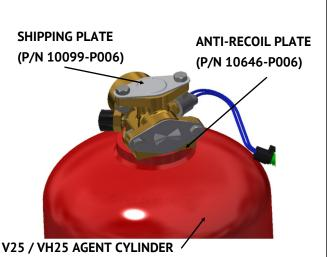
The Amerex ACT™ System agent cylinders are available in two sizes, with different mounting options and orientations. There are two different types of agent cylinders, those for use in total flooding applications and those for use in local applications. All agent cylinders are shipped fully charged from the factory. All agent cylinders are specialized DOT 4BW350 cylinders, tested to 700 PSI (4826 kPa). The operating temperature range of the cylinders is -40°F to 120°F (-40°C to 49°C).
