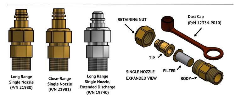
Three (3) different types of nozzles are offered for use with the ICS system as shown in the table below. Each nozzle has a specific full cone pattern diameter and range for dispersing the ICS agent to the hazard area. For specific nozzle ranges, see figure below. All nozzles used in the system are supplied with filters. All nozzles are also supplied with dust caps to prevent contamination from entering or blocking the nozzle tips. Replacement dust caps are available (P/N 12334-P010).
