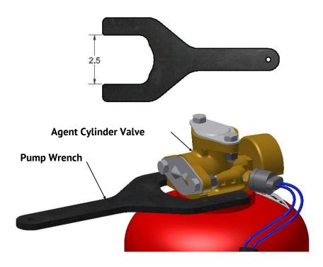
The 2 ½" Pump Wrench is used to remove or reinstall the Agent Cylinder Valve In the Agent Cylinder. It can be purchased from McMaster-Carr or other hardware supply stores. The Pump Wrench should be less than .30" in thickness for proper fit on the Agent Cylinder Valve.
