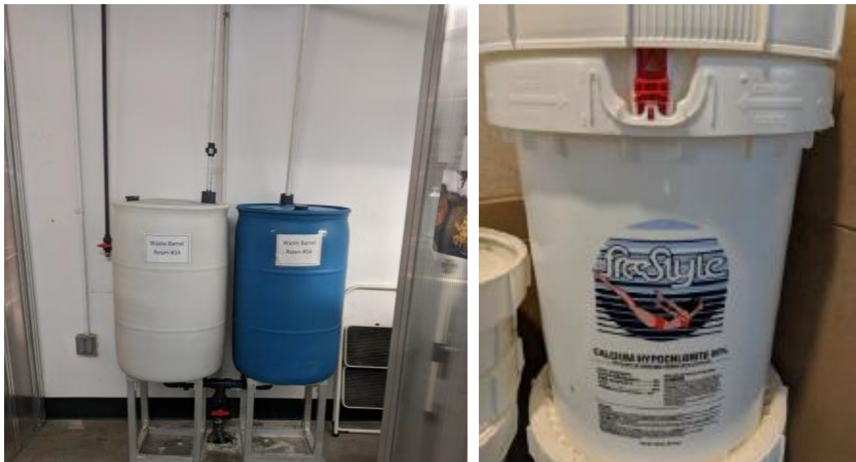
Figure 7. Wastewater vats ( left ) typical for each IAR which are treated with concentrated bleach ( right ) overnight before being disposed into the municipal sewage system.
