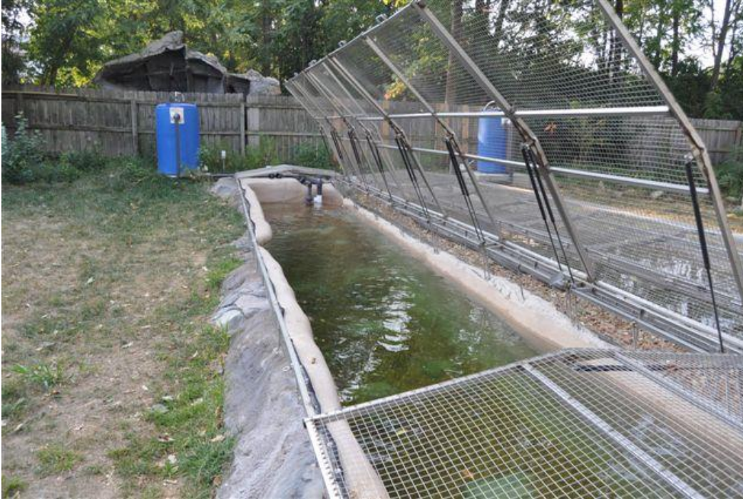
Figure 7. Hydraulic lids on stream.
