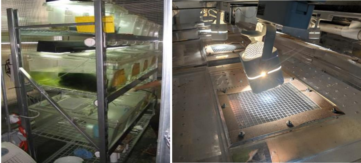
Figure 4: Left: Shelves of polycarbonate amphibian enclosures with shop lights installed typical of IARs. Right: Enclosure lids showing modifications for UV light penetration. Larger mesh can be used for larger amphibians (which feed on larger food items), but finer mesh should be used for smaller species.
