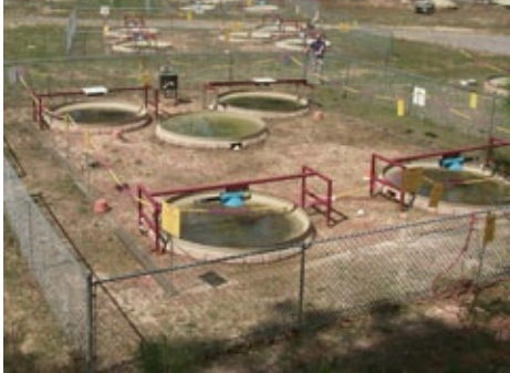
Low dose irradiation facility (LoDIF) with outdoor tanks at the University of Georgia's Savannah River Ecology Laboratory (SREL) used to exposed Scaphiopus holbrookii tadpoles. Photo: Thomas G. Hinton.
