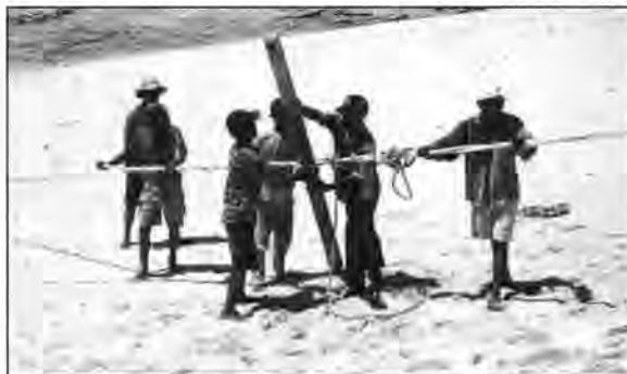
Figure XII. A Spanish windlass is used on a beach in Africa to pull a boat.
