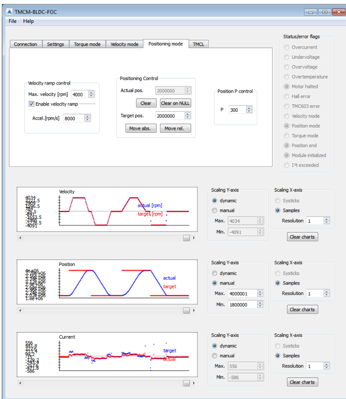
Figure 4.5 Positioning mode tab of TCMC-BLDC
