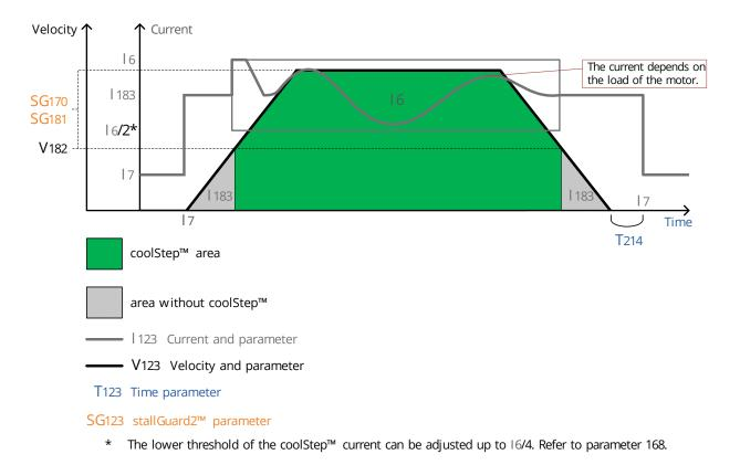
Figure 15: CoolStep Adjustment Points and Thresholds
