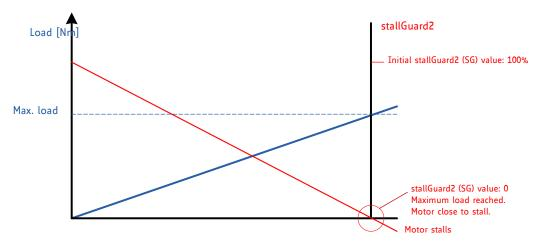
Figure 1: StallGuard2 Load Measurement as a Function of Load
