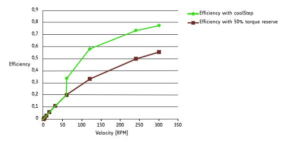
Figure 2: Energy Efficiency Example with CoolStep
