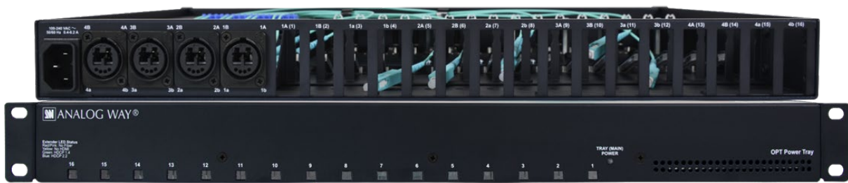
Fig. 5 - Power tray for optical extenders (ex: Neutrik OpticalCON Duo)
