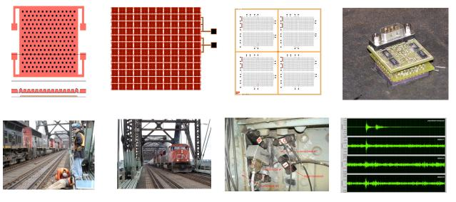
Top row, left-to-right: MEMS resonator, 125 microns across; sensor array of 144 resonators; four chips, 5x5 mm each, each chip containing four sensor arrays; newly completed system with electronics in a 35x35x30 mm volume
