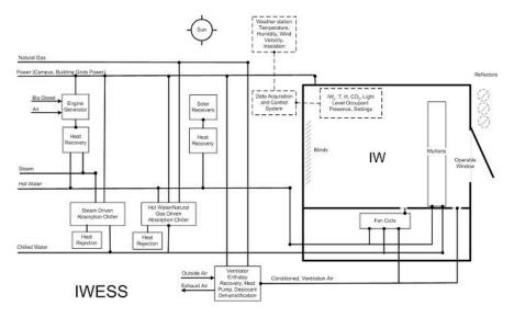
IWESS System Integrated with the Intelligent Workplace
