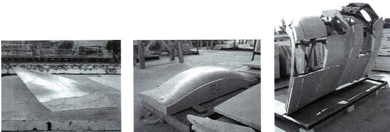
Figure 2-35 Complex shaped panel construction by CNC milling ( Left & Middle ) Milled surface panels; and ( Right ) Façade mock-up with supporting steel ribs Image after Schodek et al. (2004: pp. 62)
