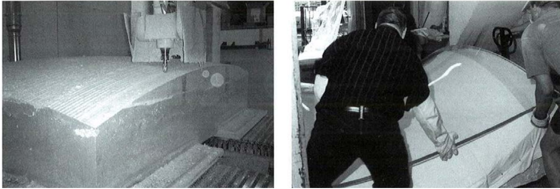
Figure 2-37 (Left) Mold milling (Right) Thermoforming acrylic sheets Image after Schodek et al. (2004: pp. 72)
