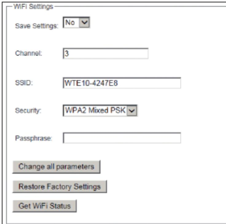
1. To change the settings, enter values into the corresponding fields for the channel used (*Channel*), the network ID (*SSID*), the encryption of the transmission (*Security*) and the WLAN password or select the respective option.
