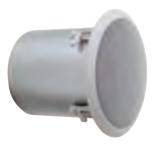
The Bogen HFCS1 ceiling loudspeaker delivers superior sound and clear intelligibility in a variety of ceiling environments. The system can be easily installed in hard-surfaced ceilings, suspended ceilings and new construction. The HFCS1 offers several levels of power output via a front-mounted rotary switch. The low-distortion speaker design, coupled with dual front exit ports, delivers high intelligibility and exceptional low-frequency response for both music and speech reinforcement.
