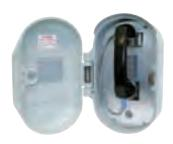
The "Tough Phone" was developed for public and industrial areas requiring a virtually indestructible telephone. Each "Tough Phone" is housed in a 1/4 in. thick, sand-cast aluminum enclosure, coated with an exterior polyurethane finish. Standard equipment includes a spring return door, 15 in. lanyard armored cord resistant up to 800 lb. of pull strength, chrome-plated keypad and proximity hookswitch. The Model 233-001 tamper-resistant screwdriver is required for installation.
