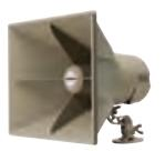
The SAH5 and SAH15 horn loudspeakers employ digital switching amplifier technology resulting in unprecedented low DC current draw and heat dissipation. This means fewer power supplies, longer cable runs and the capacity to work at higher ambient temperatures than conventional analog amplified horn speakers.
