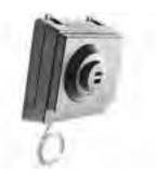
The Stinger 90 Model 196, line-powered telephone ringer provides 110 dBA output and is driven from the ringing voltage on the CO line. Rugged weatherproof housing is suitable for indoor or outdoor use. The model 196 is equipped with a three-position switch for volume control and comes with a modular cord plus screw terminals. Can be wall-mounted.
