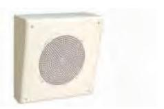
The MB8TSQ and MB8TSL speakers feature an all-steel surface-mounted enclosure with an 8 in. cone loudspeaker and multi-tap 4-watt 70V/25V transformer. The MB8TSQ is suitable for ceiling or wall mounting. The MB8TSL is designed primarily for wall mounting and its face is angled downward by 12.5 degrees.
