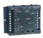
The VAR-1 is a relay device that monitors audio activity over a wide range of input voltages and operates two sets of C-Form relay contacts in response to detected activity. The VAR-1 can be used to detect voltages as low as signals directly from a microphone or as high as signals from 70 V speaker systems. A low-level output of the detected audio, transformer-isolated from the input, is also made available for use with other equipment. Also can be used as a balanced low-impedance mic pre-amp.
