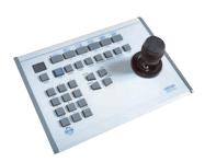
These keyboards are full-function, desktop keyboard controllers that can be used in a variety of applications. Keys select cameras and monitors; operate presets, patterns, auxiliaries and sequences; open and close the iris zoom and focus the lens; start and stop auto-frame and random scanning.
