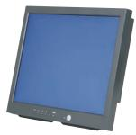
200 Series LCD monitors provide high-resolution display of VGA signals. This 19 in. monitor uses a color thin film transfer (TFT) active matrix 1,280x1,024 LCD panel that automatically adapts to the appropriate input resolution.
