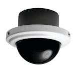
The IS150 Series Camclosure Integrated Camera System combines a camera and lens package into a small, high-security enclosure for medium-security installations subject to vandalism. The in-ceiling dome is designed for suspended-ceiling or recessed-ceiling/wall installations. An adapter plate is supplied with the dome to mount the unit to a 4S electrical box or to provide additional support for suspended-ceiling installations.
