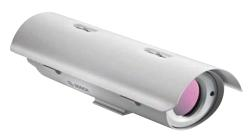
The VOT-320 thermal IP camera provides high-sensitivity, uncooled long-wave thermal images. It can tristream video simultaneously on two H.264 streams and one JPEG stream. The camera uses a Vanadium Oxide (VOx) focal-plane array with an image resolution of 320x240 pixels that delivers outstanding image quality and sensitivity. It offers a choice of various lenses - both narrow field of view (NFOV) and wide field of view (WFOV) and is available with a frame rate of 8.33 or 30 Hz.
