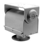
The PT570P and the PT570-24P are medium-duty pan and tilts designed for outdoor applications. Both units feature rugged worm-gear final drives to minimize backlash and prevent wind drift, and are fully adjustable for wear.
