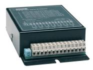
The KTD-83 is a data signal distributor that is designed for use in a Digiplex system. It is used when an RS-422 control signal must be dispersed along separate lines of two-conductor UTP cable.
