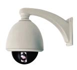
All PTZ domes include true day/night, image stabilization (except 23x) and WDR functions, are powered by 24 V AC (power adapter included) and accept RS-485 control protocol. Outdoor units include an integrated heater and an environmental shield. Pendant versions include a 1.5 in. NPT pipe coupler with ceiling flange. Actual pipe is customer-supplied.
