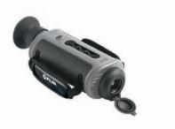
The affordable Guardsman handheld thermal imaging cameras allow security professionals to see clearly in total darkness, providing an undeniable tactical advantage. Using a 320x240 thermal imaging core, Guardsman provides four times the image clarity and detail of earlier systems while offering advanced image processing as well as grayscale and color thermal imaging.
