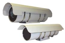
The 5 in. diameter HS9392 Series and the 7.5 in. diameter HS9396 Series Housings are designed to enclose large zoom lenses and cameras. A pressurized version is available that further reduces the amount of moisture around the electronics, and an optional pressure sensor can warn of dropping pressure within the housing. The ingress protection rating is IP67 for standard housings and IP68 for pressurized housings.
