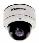
The AVxx55 series network cameras are part of Arecont Vision's full line of H.264 MegaDome IP megapixel cameras, integrating the camera, lens and housing into an all-in-one solution. Available in color or day/night versions and with 1.3 to 5 megapixel sensors, the dome cameras incorporate Arecont Vision's fully compliant implementation of H.264 (MPEG-4 Part 10) compression that uses up to 10 times on average less bandwidth and storage compared to megapixel counterparts using MJPEG compression.
