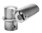
The EHXM Series explosion proof camera enclosures are designed to meet the rigorous requirements of explosion proof and dust-ignition-proof electrical equipment for installation and use in hazardous locations. The system can be installed in a standard or inverted position and features manually adjustable 200 degrees of pan and 180 degrees of tilt positioning.
