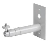
The C10-UM is a universal camera mount kit that includes all the components for wall, ceiling or T-rail clip installations for most box-type cameras with 1/4 in. x 20 in. mounting holes. The kit supports cameras weighing up to 7 lb. (3.18 kg). The ball socket of the kit allows for 360 degree pan adjustment and 90 degree tilt adjustment.
