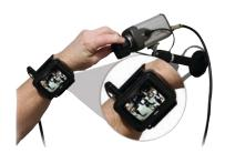
These field-friendly mobile test monitors are ideal for troubleshooting system setup/fault locations. Identify problems as they happen, see real-time data on your screen regarding performance and configuration during installation. The TM2P has a video output test pattern with color bar and gray scale chart, auto-shutoff timer,
