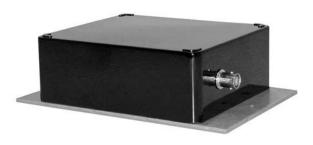
The GIT100 is a ground loop isolation transformer that reduces ground loop interference in CCTV signals and can be easily added to existing systems. The GIT100 provides a high degree of common mode isolation at power-line frequencies, but passes signal frequencies from DC to more than 200 MHz.
