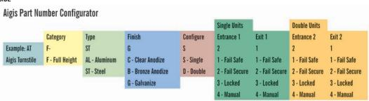
Example 1: (Single Unit) AT-FSTGS21 = A galvanized steel, single passageway turnstile with Fail-Secure entrance and Fail-Safe exit in the controlled direction(s).
