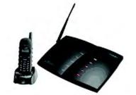
Four-line base system which is expandable up to eight base units (32 ports) and a combination of up to 90 DuraFon Pro handsets or DuraWalkie radios.
