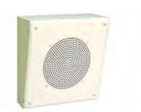
The MB8TSQ and MB8TSL speakers feature an all-steel surface-mounted enclosure with an 8 in. cone loudspeaker and multitap 4 watt 70 V/25 V transformer. The MB8TSQ is suitable for ceiling or wall mounting. The MB8TSL is designed primarily for wall mounting and its face is angled downward by 12.5 degrees.
