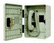
GAI-Tronics' industrial telephones are designed for those applications where standard telephones are not environmentally suitable. The auto-dial telephones are programmed to automatically dial when the handset is taken off the hook. The phones have a detachable programming keypad, preventing unauthorized tampering of the preprogrammed phone number.
