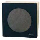
Bogen's wall baffle is ruggedly constructed of 3/8 in. particle board with reinforced corners. It is finished in simulated walnut and will house any of Bogen's 8 in. speakers. A sloping front panel provides enhanced downward dispersion. Hardware for mounting a speaker to the baffle included.
