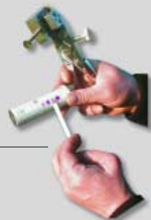
The quantity of nitrates absorbed by plants can be measured in many ways. Hand-held pliers measure the nitrate levels in plant juice to determine absorption levels.
