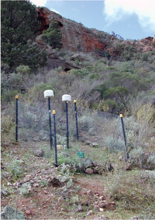
Figure 8.10 Data logging station set up at a Brachyscome muelleri translocation site to monitor climatic conditions. (Photo: M Jusaitis)
