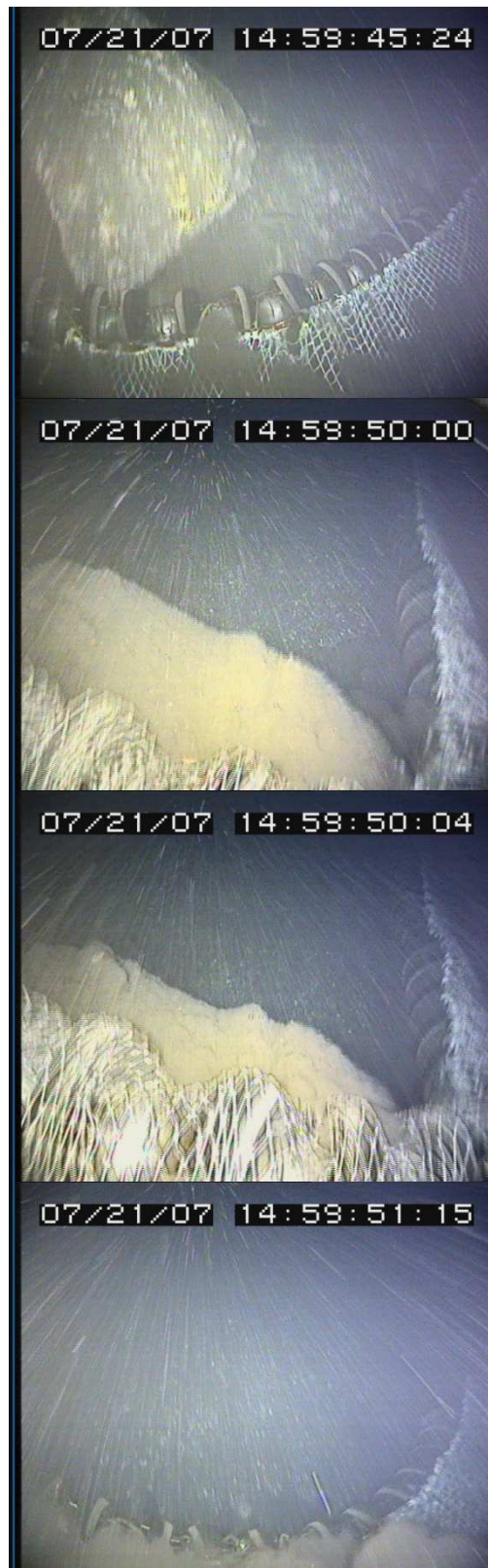
Figure A10.2. Sequence of stills taken from footage of rock-hopper ground gear of a demersal trawl distorting under tension and ultimately lifting over a large (c. 2.5 ton) rock. The rock is completely turned over during this process.
