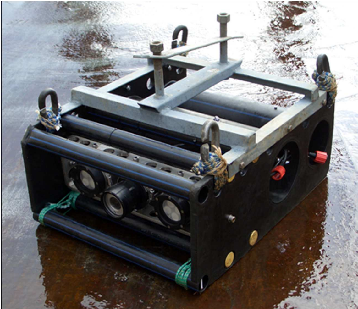
Figure A4.1. Benthic Impacts Camera System (BICS) mounted in the trawl net crash frame (with extra mounting hardware for attachment to trawl warp).
