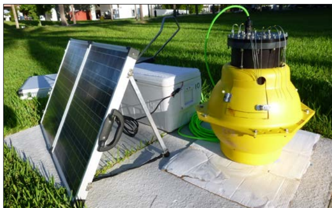
View of the autonomous ammonium instrument showing solar cell panels.
