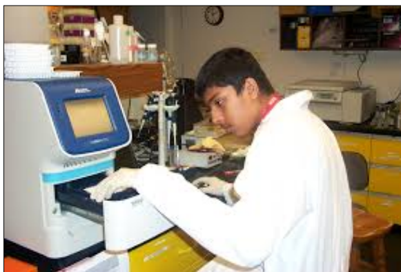
Student Intern Aditya Shetty using a quantitative real-time Polymerase Chain Reaction (qPCR) thermocycler. qPCR permits detection of fecal indicating bacteria more rapidly than traditional culture methods, and enables MST, which can identify the host source (e.g., human, bird, dog, cow) of the bacteria.
