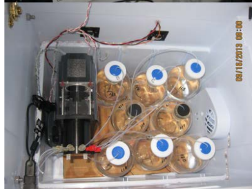
Upper: view of the instrument shows all the components of the system. Lower: inside of the thermostatically regulated cooler in which the syringe pump and eight sample bottles are housed.
